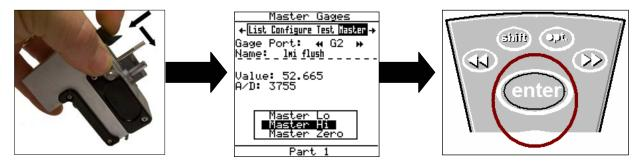
9. Place the gage in the LMI 720 master block, retract the gap peg so it will insert into the gap slot. With "Master Zero" highlighted on the collector press <enter>.
