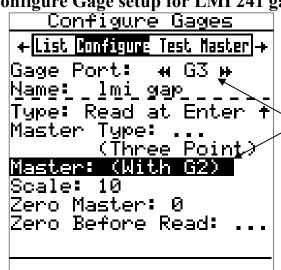
"Gage Port G3" must be matched to "Master with G2" to calibrate both flush and gap at the same time.
