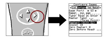
The "Configure Gages" screen needs to be set as follows. Failure to set this screen properly 14. may cause undesired results. The top screen shows a standard LMI 241 configuration, the bottom screen shows a standard 241-B configuration.
