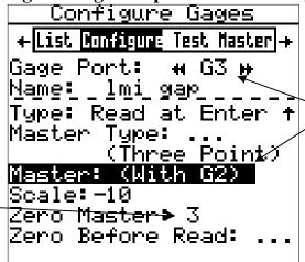
"Gage Port G3" must be matched to "Master with G2" to calibrate both flush and gap at the same time.
