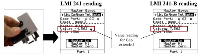
7. Retract the gap peg, observe the value in the "Master Gages" screen of "Gage Port G3" in the collector.
