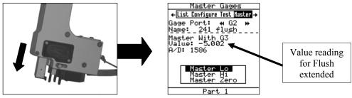
2. Retract the flush tip, Observe the value in the "Master Gages" screen of "Gage Port G2" in the collector.
