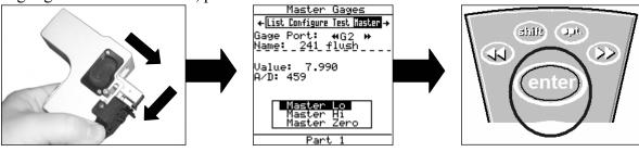
8. Fully compress the flush tip and extend the gap finger of the LMI 241BWV2. With "Master Hi" highlighted on the collector press <enter>.
