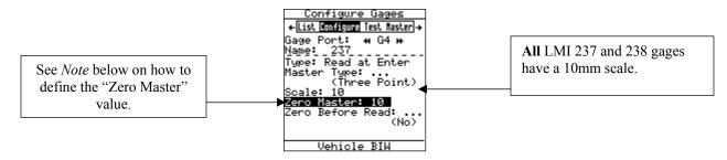
Note: The ZERO MASTER is the constant value or offset in the inspection range specific to the LMI Ultra Mini Seal Gap Gage. The collector will add the ZERO MASTER value to the dynamic reading from the gage and display an actual reading on screen.
