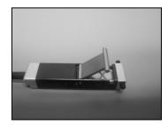
9. Advance to MASTER ZERO and place the Ultra Mini Seal Gap Gages on a certified flat surface (LMI 3030 or 3062 works well) and press the <Enter>button on the keypad.
