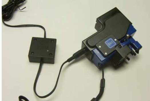
Fig. 3.12 SK5155 In-Line Charger plugged into gauge
