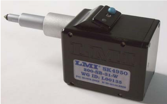
Fig. 3.1 LMI 200 Wireless Probe
