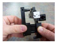
2. Slide the striker pick-up slide over enough to allow the taper pin to engage the slide.
