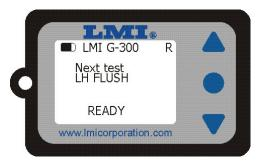
The routine is set in the within the gage. This is created and downloaded from the UGI software package. Refer to UGI Manual for test routine setup. For this example, the partfile has four points: LH Flush, LH Margin, RH Margin, and RH Flush.
