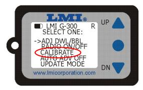
With the gage fully extended, press the PB button to take the "Cal LO" reading.
