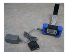
*Note:* The SK5487 Bumper to Box Gage does not have an On/Off button. The gage will go into a low power "sleep" mode after 5 minutes of no activity, but will continue to draw a minimal
