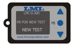
As indicated on the screen, press the "PB" button to start a new test routine. This screen will appear whenever a new test start is required. The screen flashes so that the operator knows to go to the first test point in the sequence.
