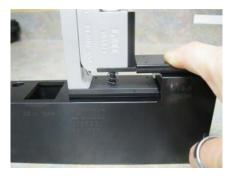
The screen will advance to Gap Master (G Cal Master). Place the gage onto the SK5523 Master Block, in the 26mm Gap position, and then press the PB Button.
