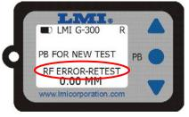
The gage will automatically advance from each Flush and Margin position. At any time during a routine, pressing the "UP" or "DN" buttons will move the user forward or back in the test routine in the event that the operator wants to retake a test point.
