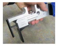
The screen will advance to "Cal HI". Fully retract the gage and then press the PB Button.
