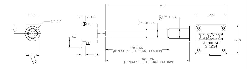
9.5 MM DIA. ON TRANSDUCER BARREL FITS LMI 261 AJDJUSTABLE THREADED BUSHING OR ANY STANDARD 3/8" ID BUSHING
