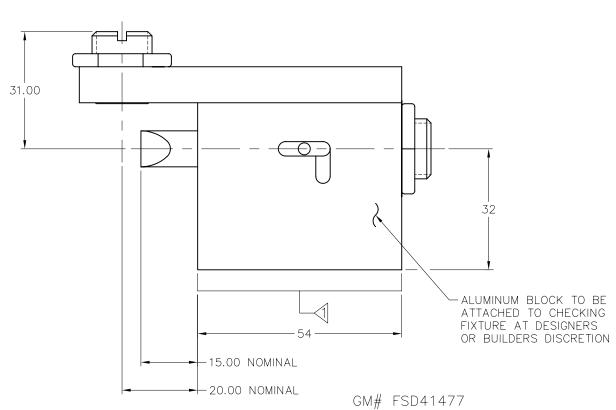
BRACKET SHOWS ALLOWABLE AREA FOR BOLT HOLE PATTERN AND DOWELING.
