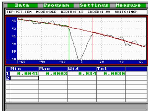
**Measurements** - The depth (Min) of a scratch is measured from its deepest point relative to a line-fit of the two adjacent surfaces. Material pushed out of the scratch and creating a surface point above the line-fit is also measured (Max).
