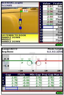
Routine Mode – Routine mode allows the user to run inspection routines developed using the LGWorks software. Multiple routines can be stored on the controller and automatically opened with the entry of an associated VIN, trace number or other identifier. Graphical and text instructions guide the operator to the proper measurement locations. Color-coded results and audible tones alert the operator to out-of-spec conditions.
