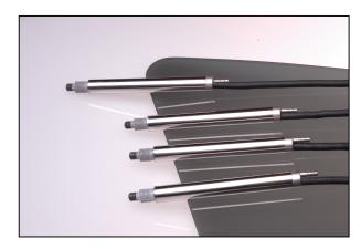
LMI 5300 probes extend to meet the part when air is supplied to the probe. Each probe has a 10mm range of travel with an accuracy of +/- .03 mm. Each probe has five main components:
