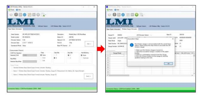
With Wireless Utility open, Press and release the in/mm to send the information over to Wireless Utility. This will cause Wireless Utility to move from the Base Station Information screen to the Gauge Info screen
