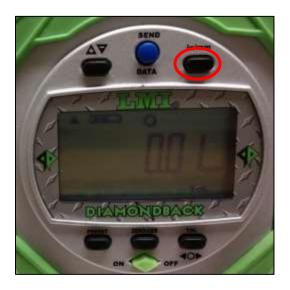
Place the gauge into Setup Mode by pressing and holding the in/mm button for about 4 seconds until SETUP is shown on the screen.
