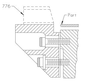
HOLES TO BE REAMED BY USER FOR A 3.18 DIA DOWEL
