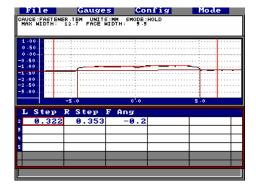
LaserGauge System - Depending on the diameter of the fastener and the resolution required, an HS300 sensor with either a .50" or 1.2" field-of-view is recommended. An LG1102 controller allows the operator to view the profile of the fastener and make sure that it is centered in the display for the best measurement.
