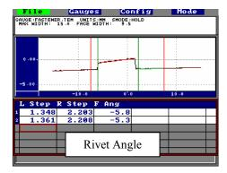
**ANGLE** - The angle of the head of a rivet, screw, bolt or other fastener relative to adjacent surfaces may indicate improper installation. Even though the head is within flushness tolerances, an exaggerated angle can be of importance to aerospace and space vehicles.
