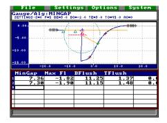
Measurements - Measurement methodology is defined in software, not hardware, and flexible Virtual Gauges can be used with different settings to simulate almost any measurement method imaginable. Once selected, Virtual Gauges run automatically on the LaserGauge and can return measurements using caliper, minimum gap, nearest point and other virtual methodologies.
