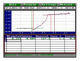
Measurements - The laser weld algorithm calculates the mismatch between the two sheets, weld concavity and weld convexity in both absolute terms and as a percentage of a sheet thickness and it identifies any undercut at the edge of the weld. All of the measurements are made automatically when the sensor trigger is released. Parameter tolerances are entered only once at the beginning of an inspection session and any out-of-spec conditions encountered are displayed in red.
