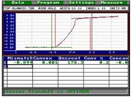
LaserGauge System - Due to the narrow width of the laser weld and the resolution required, an HS400 sensor with a 0.150" field-of-view is used. An LG1102 controller provides the graphical feedback necessary to allow the operator to position the laser stripe over the weld at a designated location and to view the profile as the measurements are being made.
