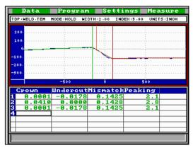
**LAP WELD** - A weld joining overlapping panels creates similar characteristics to the laser weld. There should be no mismatch in the panels other than the height of the panel that is placed on top.
