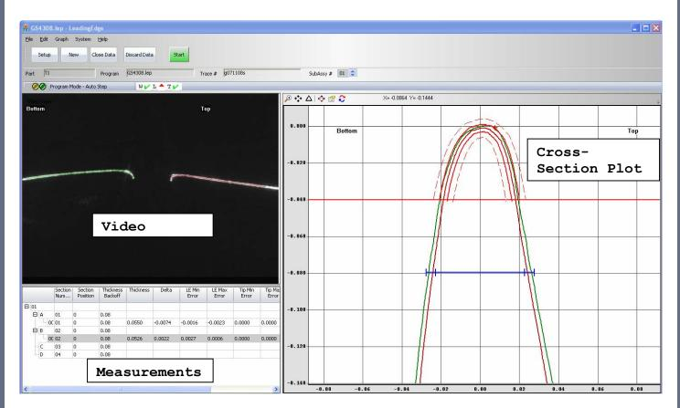
**Documentation** - Data displayed in the table can be saved as documentation of the measurements. A scan or profile can also be saved to a file. The file is a flat tabular file with x,y,z coordinates of each point in the scan; the x value representing the position along the blade.
