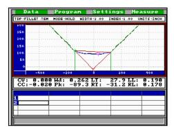
**FILLET WELDS** - Fillet welds are used when two panels are joined at a 90° angle to each other. Since the only thing visible to an inspector is top surface of the weld between the two panels, there is practically no manual or mechanical means of measuring parameters of a fillet weld.
