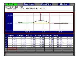
LaserGauge System - A sensor that has a field-of-view that is two to three times the nominal width of the weld bead is recommended. For welds other than very small laser-welds, an HS300 series sensor with a 0.50", 1.2" or 2.4" FOV is recommended. The LG1102 controller provides a graphical display of the surface profile of the weld as the measurements are being taken.
