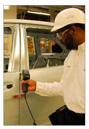
**Operator Feedback -** Three LED's at the front and the rear of the sensor direct the operator to roll the sensor to the correct angle before the scan is completed. A 2 x 16 LCD is used to display messages, alerting the operator of scanning errors, indicating when a good scan has been completed, showing the measurement value, and providing instructions on where the next measurement is to be taken.
