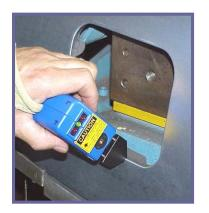
**Trigger -** Low-tactile trigger buttons are located on either side of the sensor. Either button can be used as the trigger, depending on the preference of the operator.
