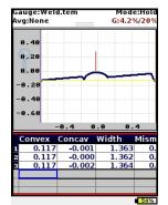
fastener or weld algorithm. Measurements can be made in millimeters or in inches. Multiple measurements are calculated on each scan and values are displayed in the data table. Values are color-coded to indicate in-spec and out-of-spec conditions.
