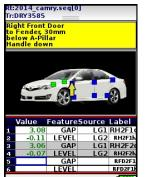
The routines are developed using the LGWorks software, and the routine files are sent wirelessly to the sensor through a ZigBee module or by using a USB cable.
