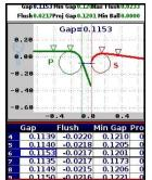
the fastener or weld algorithm. Measurements can be made in millimeters or in inches. Multiple measurements are calculated on each scan and values are displayed in the data table. Values are color-coded to indicate in-spec and out-of-spec conditions.
