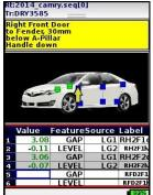
A routine is started when the operator enters the identifying number for the assembly, or the optional barcode reader can be used to scan the identifier, such as a VIN. Operators follow graphical instructions to position the sensor at predetermined measurement locations, and the appropriate measurement algorithm is loaded automatically.
