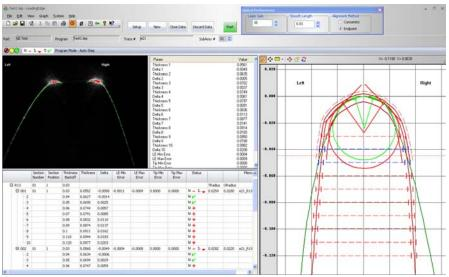
**Programs** – Separate programs can be developed for different blades, specifying different profile nominals and templates and different setback distances for thickness measurements.
