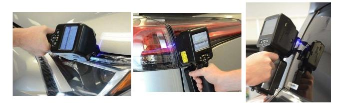
Routine and Gauge Modes – Inspection routines developed using the LGWorks software can be run directly on the sensor. Detailed graphics and on-screen messages guide the inspector from one measurement to the next. Complex calculations referencing measurement data can be processed in the routine and included in the data file.
