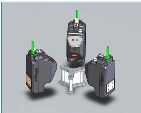
**Standoffs** - Since mechanical standoffs are used only to bring the sensor into an optimal depth-of-focus position, standoffs are not necessary for applications where the sensor is mounted to a fixture or robot. Positioning the sensor at the optimum distance from the part can be designed into the fixture or can be controlled robotically with feedback from the scan.
