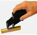
**Radius** – A radius stamped into the part and the location of the radius relative the part's edge, called the flange, must be precise for fit-up and aesthetic reasons. Small inside radii are almost impossible to measure with mechanical radius gages. An inspector cannot always see the fit of the template gage against the sheet metal because of the design of the part.
