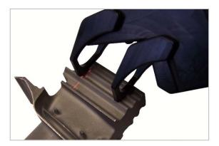
angled panels, edges with large radii and closure seals in the gaps. Mechanical devices struggle to measure gap and flush features on such complex surfaces.
